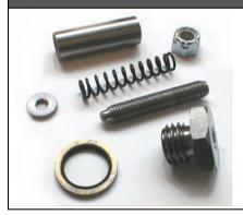
It is essential to maintain correct timing chain tension for your engine to run reliably. Unfortunately the tensioner plunger assembly can often become seized making chain tension impossible to adjust. Our tensioner kit includes a tensioner plunger, spring and screw as well as a housing nut and seal allowing you to replace a seized plunger assembly and ensure correct timing chain tension for a reliable engine.
