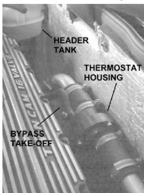
Alternatively there may be a short section of hose, connected to an aluminium pipe, running parallel to the cam cover. In these cases the aluminium pipe will need to be shortened and the thermostat housing fitted inline with additional large bore hoses (not included in the kit).
