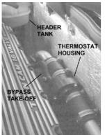
Alternatively there may be a short section of hose, connected to an aluminium pipe, running parallel to the cam cover. In these cases the aluminium pipe will need to be shortened and the thermostat housing fitted inline with additional large bore hoses (not included in the kit).
